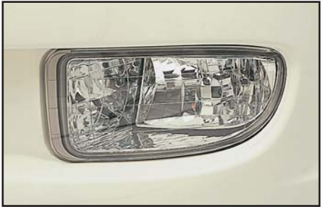
Fog Lamps Enhance vision at night, or in inclement weather.
