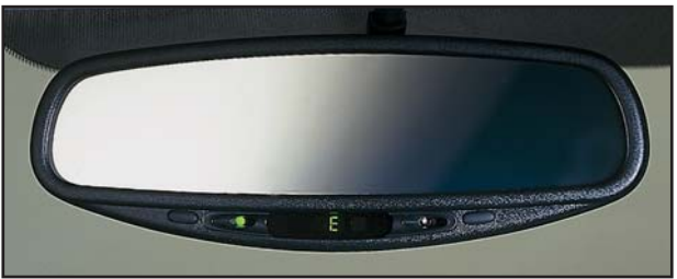
Auto-dimming Mirror / Compass Includes electronic compass. Mirror darkens when head-lights are detected from rear of vehicle. Early production vehicles may require additional harness.
