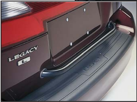
Rear Gate Bar Mounts to rear wagon door for easier opening and closing.
